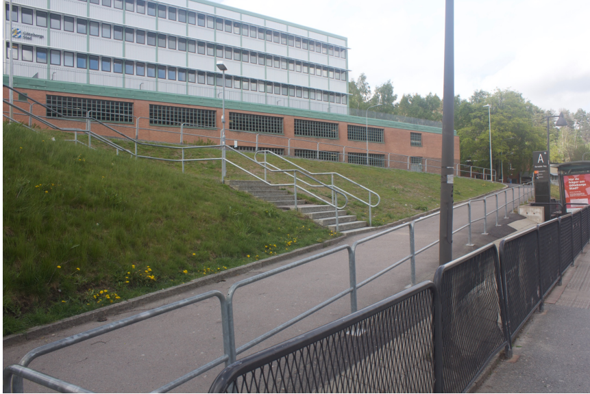
Picture 11. Steep walkway from stop for wheelchairs, shorter stairs for pedestrians. Photo: Per Olof Larsson
