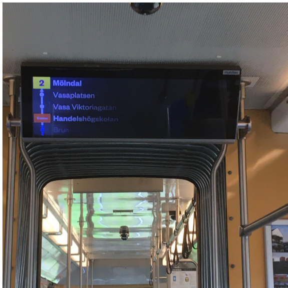
Picture 21. Faulty display. The right side is dark. Photo: Per Olof Larsson
