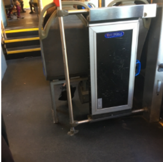
Picture 8. M31 tram, with manual ramp and stairs up to high-floor section. Photo: Per Olof Larsson
