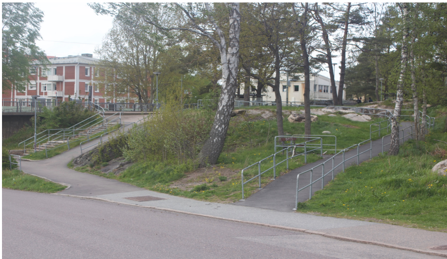
Picture 12. Three routes from the stop. A short one for pedestrians, a very steep one for, e.g. prams, and a very long one for wheelchairs. Photo: Per Olof Larsson
