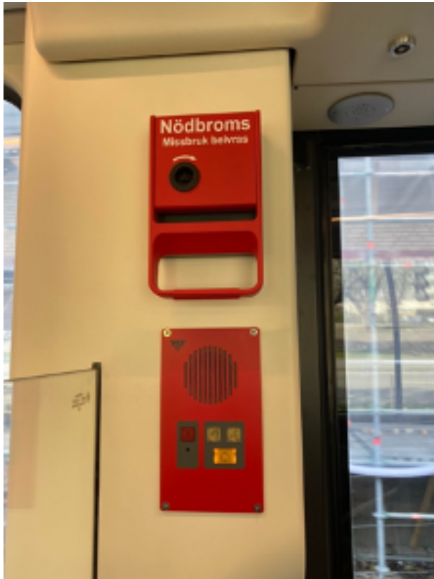
Picture 20. M33 tram, emergency brake that cannot be reached by a wheelchair user. Photo: Robert Kindberg
